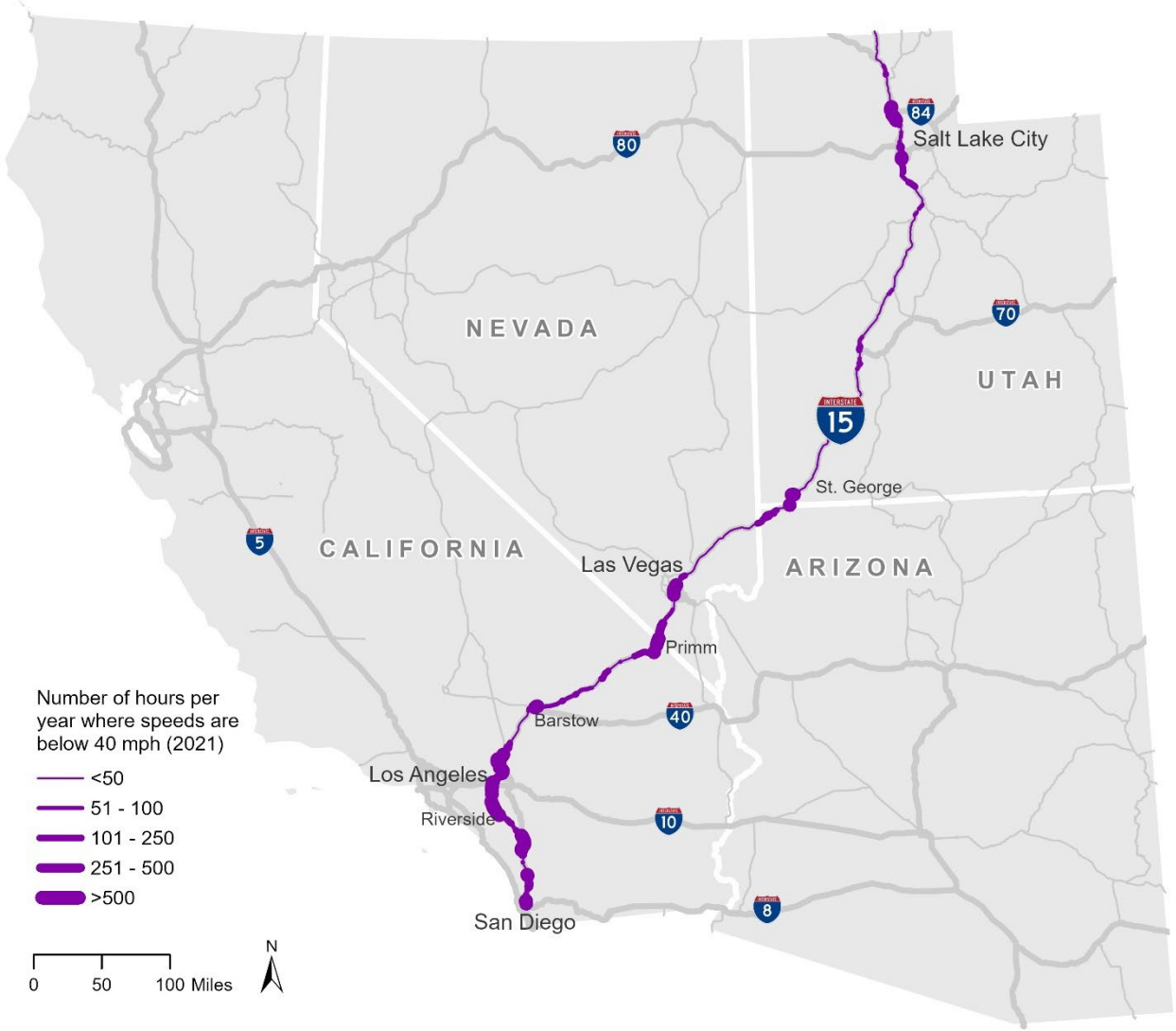
Figure 4.14 I-15 Interregional Severity of Chokepoints: Total Number of Hours where Speeds are Below 40 mph
